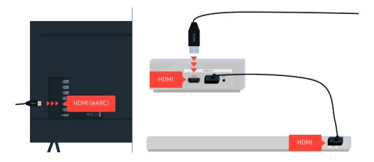
If your Sound Bar is connected to a receiver, and the receiver is connected to the TV using an HDMI cable, check the HDMI connector on the back of the TV. The cable must be connected to the HDMI (eARC) port on your TV.
