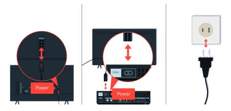
First disconnect and reconnect the power cables and HDMI cables on the back of your TV or the One Connect (OC) Box, then unplug the power cable and plug it back into the wall outlet.
