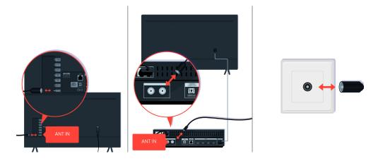
Check the antenna and input cable connections.
