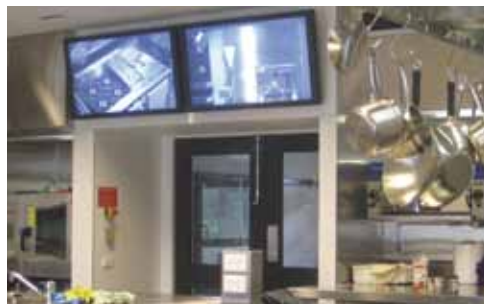
Two LCD screens side by side to display food preparation area and stove top in full HD
