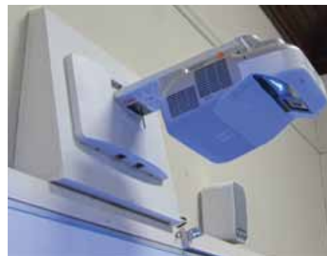
The EPSON EB 475 Wi mounted on an angled wall bracket to overcome the issue of the slanting projection surface
