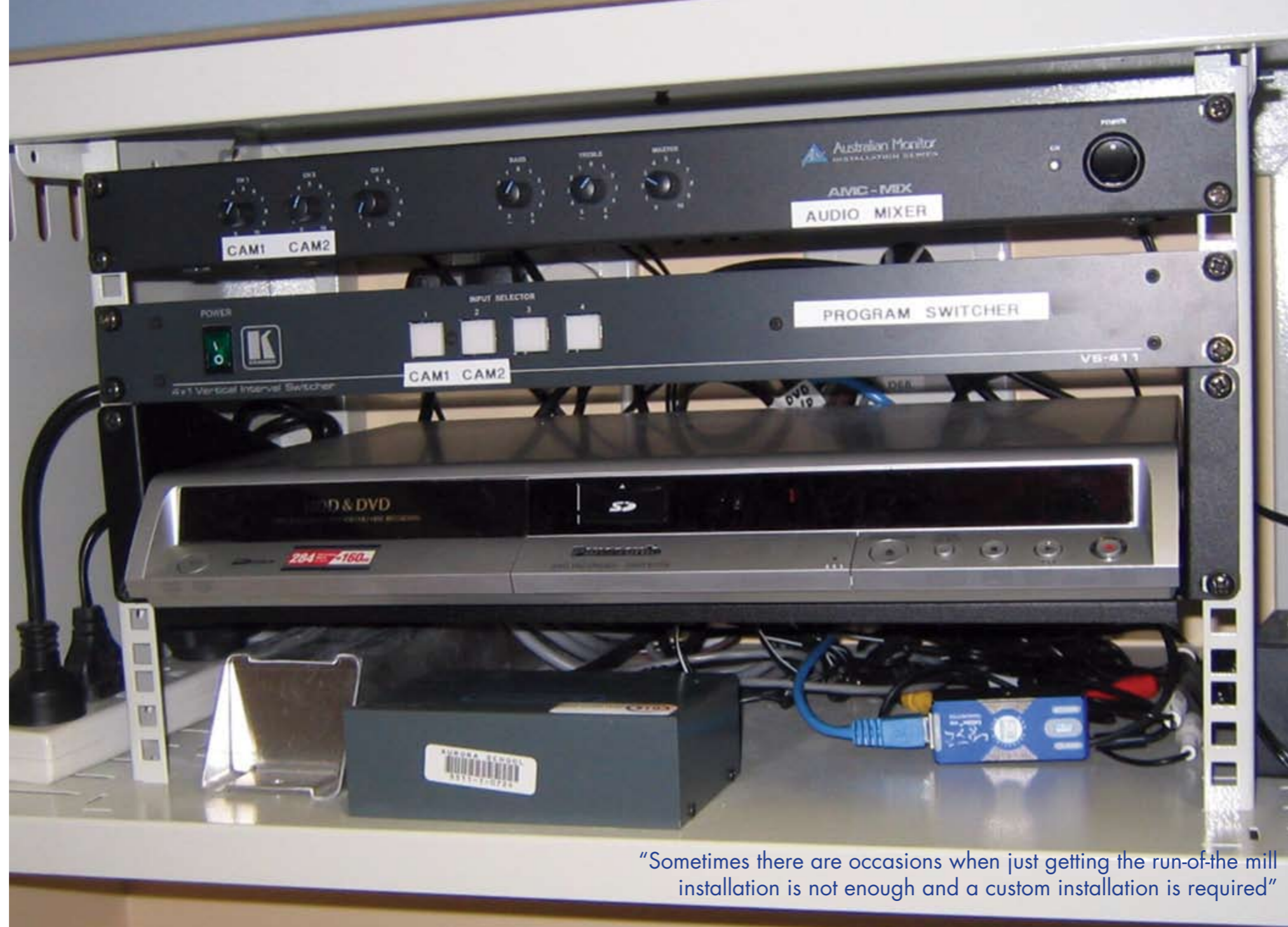
ABOVE: 6RU rack that houses equipment including the switcher and Panasonic HDD/DVD recorder that is used by staff for local burning or further routing to the DVC Capture server.
