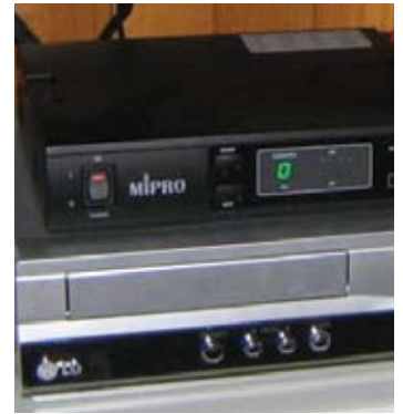
ABOVE: Mipro UHF 16 channel receiver, automatically detects the best channel, providing clear reception every time
