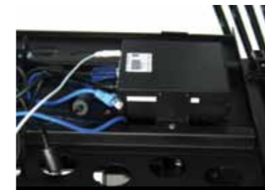
ABOVE LEFT: A small AOpen PC fitted to the rear of the ceiling mounted 42" Panasonic Professional Plasma panel facilitates a wide variety of digital signage application.
