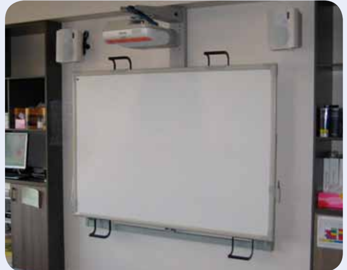
ABOVE: Height adjustable interactive whiteboard and projector facilitates easy use by students for more inclusive learning
